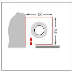
Type B: BX = 350 mm, BW = 260 mm Type C: BX = 190 mm, BW = 290 mm Type D: BX = 290 mm, BW = 360 mm Type E: BX = 380 mm, BW = 420 mm
