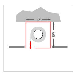
Type A: BX = 285 mm, BW = 200 mm Type B: BX = 350 mm, BW = 260 mm Type C: BX = 190 mm, BW = 290 mm Type D: BX = 290 mm, BW = 360 mm Type E: BX = 380 mm, BW = 420 mm
