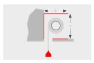
**Type A:t** 380 mm, **h** 350 mm **Type B:t** 460 mm, **h** 430 mm
