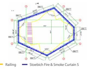
Product: Installation type: Fire rating: Manufacturer: Stoebich Fire & Smoke Curtain S Room creating textile fire protection closure which runs around the corner 2 hours Stoebich Fire Protection
